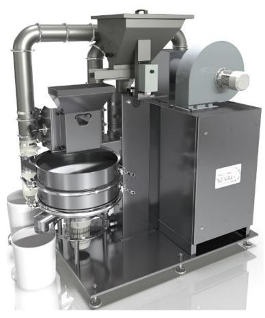
Inlet production capacity: up to approx 30-40 kg/h referred to roasted cocoa beans.
